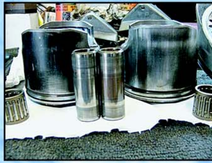
The parts that came out of Williams' test sled showed no traces of oil residue. They also showed no traces of wear for an engine with 2,000 miles on it.
