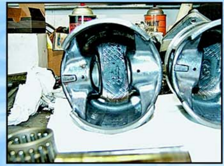
The parts that came out of Williams' test sled showed no traces of oil residue. They also showed no traces of wear for an engine with 2,000 miles on it.
